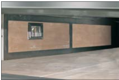
Deck side in refractory material
